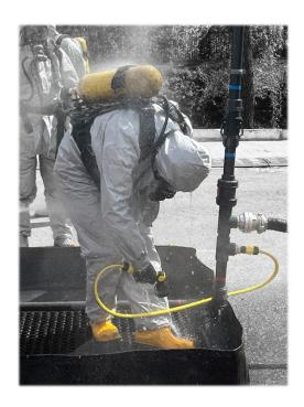
The Decontamination frame DC-1P is designed for conducting special and sanitary treatment of emergency services personnel in the event of chemical, biological, or radiological incidents.
